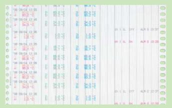
Printing of measured values at intervals of 10-60 minutes. Note: Analog trace is not available for logging printing.
