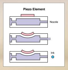
The ink jet mechanism is formed on a thin silicon chip (17.6 x 16mm) using silicon micro machining technology. It is provided with piezo elements.
