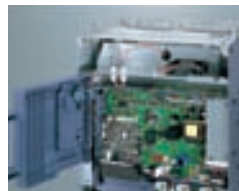
The inverter's mounting screws and power connector can be removed from the front.
